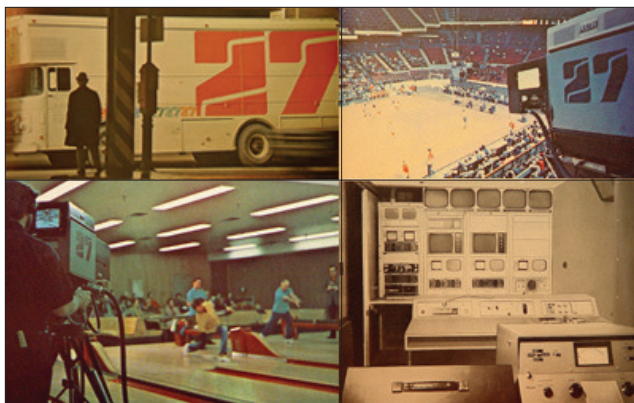
Figure 3.12 Some stations shared cameras and other production gear for inside and outside productions by putting gear on wheels. This video operator's position supporting three RCA TK-44 cameras was on wheels so that it could be wheeled into a rental truck for remote productions for a PBS station in the early 1970s.
