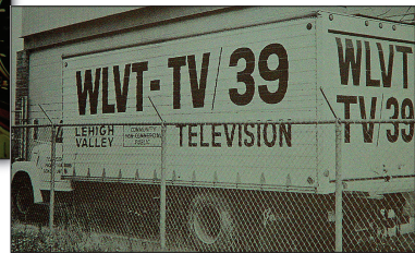
Figure 3.16 This truck was not only used for remote production, but was also the production control room for this PBS station when the truck was in port (parked at the station). A "jetway" connection hall ran from the building into the truck. A number of large stations used this approach, such as KTVU, Oakland-San Francisco.
