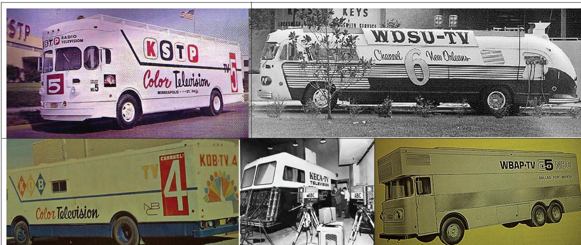
Figure 3.5 Many local television stations had their own large trucks. Before ENG and EFP, simple television production on location often took vehicles that were 35 feet long. The infrastructure to take two television cameras into the field wasn't much more than to take just one, so multiple-camera trucks were the norm. The problem was that the infrastructure for that first camera was enormous by today's standards. Standard complement was two black-and-white cameras (KECA — later KABC), four black-and-whites (WDSU), or a combination of two color and four black-and-whites (KSTP and KOB). The most ambitious was six color cameras (WBAP), but this was on a late 1960s truck, while the KECA van was 20 years prior. Of the trucks shown, only KOB (also a late '60s truck) and the WBAP truck carried VTRs. KOB had one, and WBAP carried two, which was impressive for the time.
