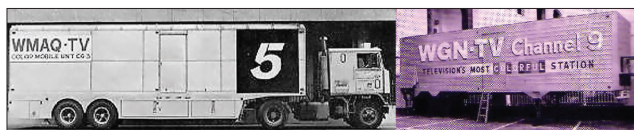
Figure 3.8 Two tractor-trailer units used by Chicago television stations in the '60s and into the 1970s. The tractor-trailer unit allowed the equipment compartment to be separate from the vehicle drive. Trailers allowed for more equipment and people space than a step-van, or box-cab vehicle. Because the tractor-trailer unit could carry more, it weighed more, resulting in more regulation of the truck and more costs.
