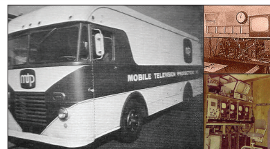
Figure 3.6 Another Gerstenslager truck with an original configuration that included four black-and-white cameras. The mid-1960s saw the addition of a two-inch VTR and a vidicon camera to shoot the output of a slide projector, approximating a crude film chain.
